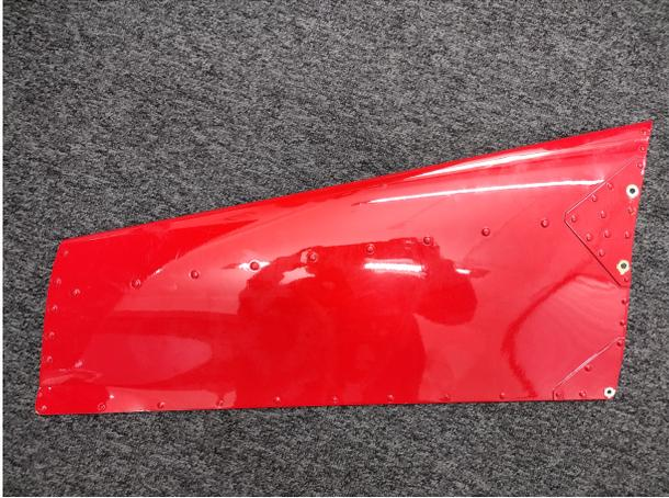
Figure 11: Top down view of the Helicopter Stabiliser wing showing the spanwise direction and shape.
