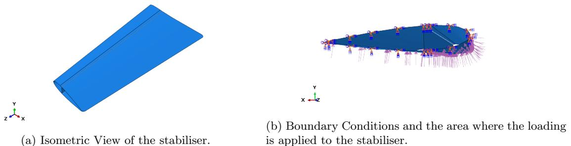
Figure 1: The different views of the geometry representing the stabiliser in the Abaqus Software.
