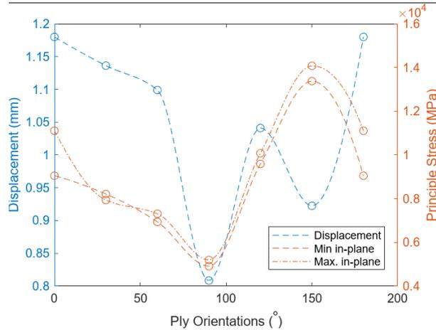
Figure 3: The effect of different fibre orientations on a single-ply composite on the deflection of the stabiliser tip under the spar.
