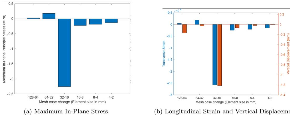
Figure 2: Mesh Convergence test for the Longitudinal Strain and the Vertical Displacement measured consistently at the same point for each of the different mesh size cases.
