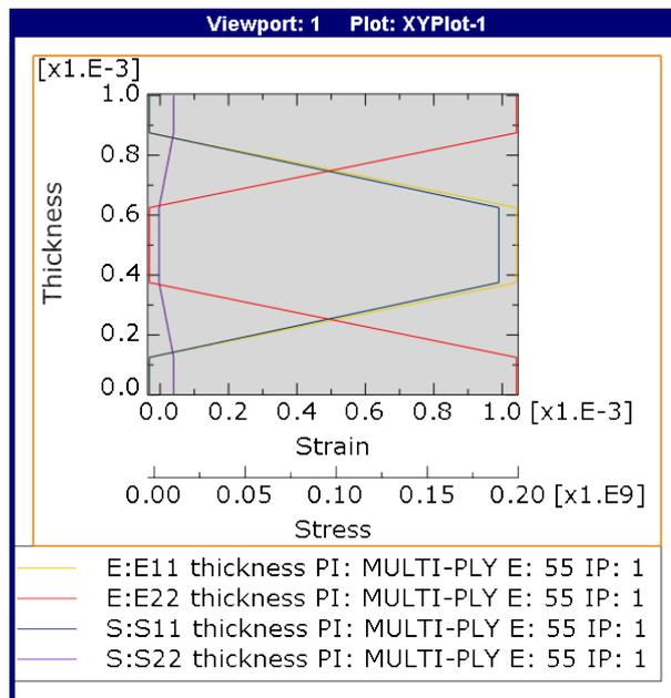
Figure 5: A plot of the stresses and strains throughout the layers of the ply model used in the Abaqus Model. Each layer is 0.25mm thick.
