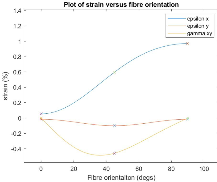
Figure 4: Comparison between the theoretical calculations shown by the lines on Matlab compared to the 'x' values which show the points of data from Abaqus.
