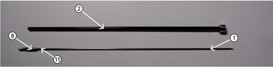
Figure C.1: A top view of the two main sections to the Scissor attachment. It is labelled with each of the parts that have been made in SOLIDWORKS. The features of the parts can be seen in the Bill of Material in Table 3.1
